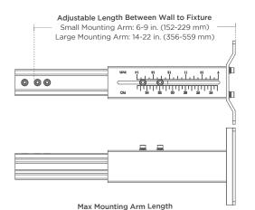
Small Mounting Arm: 10 in. (254 mm) Large Mounting Arm: 23 in. (585 mm)
