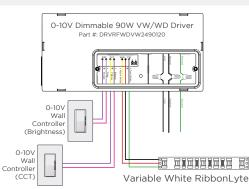
Note: 2-Channel 0-10V Dimming maintains a consistent light output level while changing color temperatures.
