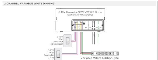
Note: 2-Channel 0-10V Dimming maintains a consistent light output level while changing color temperatures.
