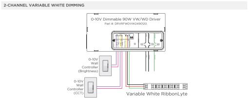
Note: 2-Channel 0-10V Dimming maintains a consistent light output level while changing color temperatures.
