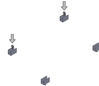
3. Push the Neon Apex into place in the mounting clips and make all necessary electrical connections. All wires should be exposed, and the product is sealed. Do not cut the channel or remove end caps.
