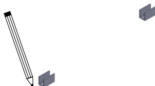
2. Drill pilot holes and then fasten the mounting clips to the surface using the screws.
