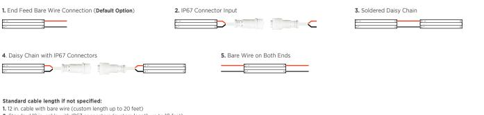
2. Standard 12 in. cable with IP67 connectors (custom length up to 10 feet)
