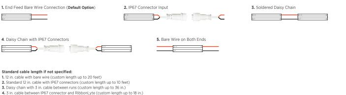
3 in. cable between IP67 connector and RibbonLyte (custom length up to 18 in.)
