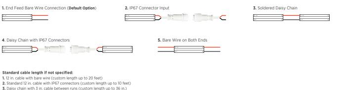
4. 3 in. cable between IP67 connector and RibbonLyte (custom length up to 18 in.)
