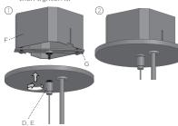
2. Attach the Cross Bar (G) to the Junction Box (F) with screws, & insert the screw into the hole in the center of the Cross Bar (G).
