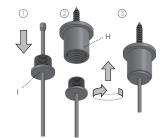
6. As an added precaution, make sure the coupler is tightened to the fixture securely.
