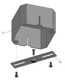
5. As an added precaution, make sure the coupler is tightened to the fixture securely. Adjust the cable length to desired height on top of the fixture, and cut excess cable off.
