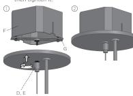
2. Attach the Cross Bar (G) to the Junction Box (F) with screws, & insert the screw into the hole in the center of the Cross Bar (G).
