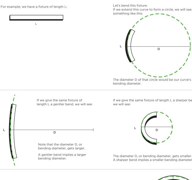
We define a fixture's minimum bending diameter because of this relationship; some of our fixtures are limited by the sharpness of the specified bend. A fixture's minimum bending diameter defines the sharpest curve it can make without jeopardizing the integrity of the LED performance.
