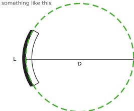
The diameter D of that circle would be our curve's bending diameter.
