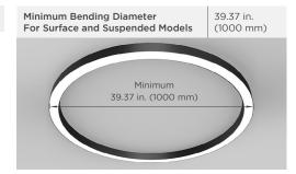
**WARNING:** DO NOT bend fixture past the listed minimum bending diameter. Defects caused by over-bending will result in a voided warranty.
