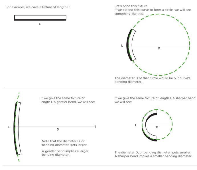
We define a fixture's minimum bending diameter because of this relationship; some of our fixtures are limited by the sharpness of the specified bend. A fixture's minimum bending diameter defines the sharpest curve it can make without jeopardizing the integrity of the LED performance.
