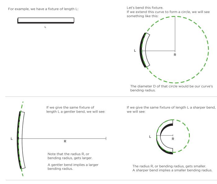
We define a fixture's minimum bending radius because of this relationship; some of our fixtures are limited by the sharpness of the specified bend. A fixture's minimum bending radius defines the sharpest curve it can make without jeopardizing the integrity of the LED performance.
