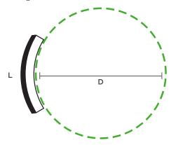
The diameter D of that circle would be our curve's bending diameter.
