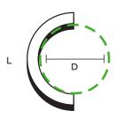
The diameter D, or bending diameter, gets smaller. A sharper bend implies a smaller bending diameter.
