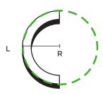
The radius R, or bending radius, gets smaller. A sharper bend implies a smaller bending radius.
