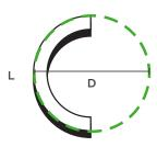
The diameter D, or bending diameter, gets smaller. A sharper bend implies a smaller bending diameter.
