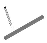
6. Drill pilot holes, then fasten the Mounting Channel to the surface using screws.
