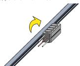
6. Cut wires to fit. Cap end wires.
