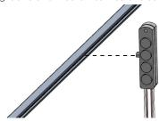
**4.** Rotate module clockwise until Turn Lock pin locks into place, parallel with I-Beam.
