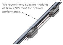
**7.** Attach to power supply. For best results, be sure to balance load to the power supply. Please reference Power Supply Loading table on page 2.
