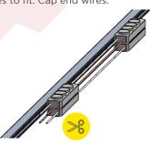
\* When using Mounting Bracket, cut Retrofit bar to rough size of opening and adjust with Mounting Bracket. When using clear end caps to fit in existing brackets, cut Retrofit bar to these lengths to match 11 standard fluorescent lengths.
