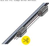
\* When using Mounting Bracket, cut Retrofit bar to rough size of opening and adjust with Mounting Bracket. When using clear end caps to fit in existing brackets, cut Retrofit bar to these lengths to match 11 standard fluorescent lengths.
