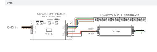
DMX WIRING DIAGRAM - COMPATIBLE WITH ALL MODELS OF VARIABLE WHITE RIBBONLYTE
