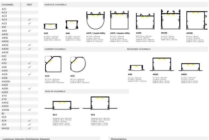
/+180 -150 150 -12 120 -90 60 UNIT:cd CO/180,123 C90/270,119.3 150 AVERAGE BEAM ANGLE (50%) :121.5 DEG
