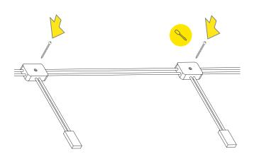
4. Connect OptiRayz rigid light bars to wire harness. (Daisy chain extra light bars or trim to fit at available cut points as needed.)
