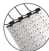
Daisy chain up to 10 full sheets with jumpers
