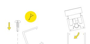
2.) Rotate fixture into bracket.
