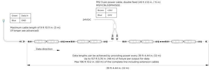
39 ft 4.44 in. (12 m) Note: Lengths longer than 19 ft 8.22 in. (6 m) need power input from the middle
