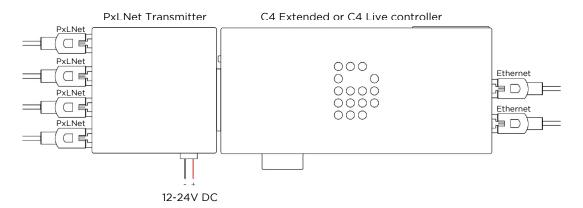
IMPORTANT: The C4 controller needs power separately. This is done with a separate DC power jack cable.
