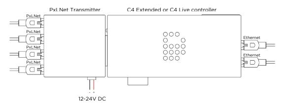
IMPORTANT: The C4 controller needs power separately. This is done with a separate DC power jack cable.
