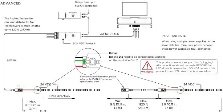
The C4 Live controller provides data output up to 37 ft (11.3 m) per output
