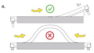
Slide Nano Flex fixtures into mounting clips/channel starting from one end. DO NOT start in the middle. DO NOT try to stretch Nano Flex fixtures.
