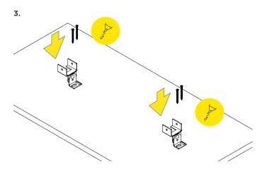
Affix adjustable mounting brackets to mounting surface with screws.
