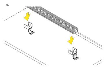
Place asymmetric channel fixture into adjustable mounting brackets.
