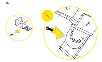
Adjust angle of adjustable mounting bracket and lock in position by using small screw.
