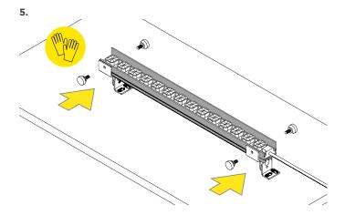
Hand-tighten screws to secure sides of the adjustable mounting brackets and lock the channel in place.
