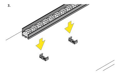
Place asymmetric channel fixture into mounting brackets.
