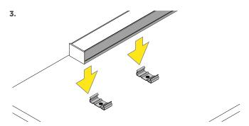
Place symmetric channel fixture into mounting brackets.
