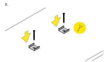
Affix mounting clips to mounting surface with screws.
