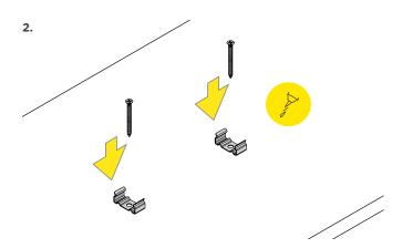
Affix mounting brackets to mounting surface with screws.
