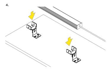
Place symmetric channel fixture into adjustable mounting brackets.
