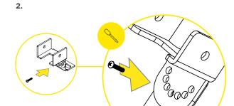
Adjust angle of adjustable mounting bracket and lock in position by using small screw.
