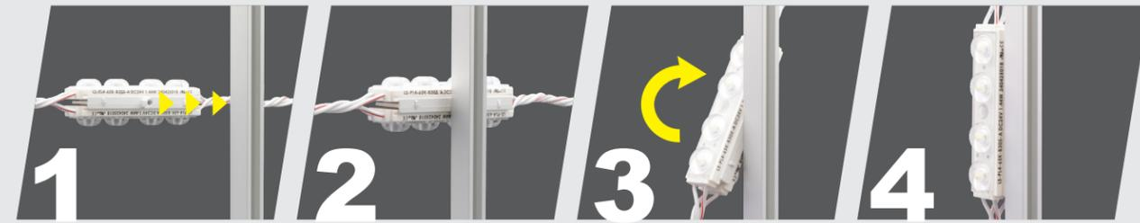
> Turnlock PRO System locks LEDs firmly in place
