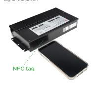
5. The App should then show the "Writing Drivers" page. Press the "Output setting" tab at the bottom of the screen. In the "DALI bus" row, toggle DALI bus power ON. (The slider should move from left to right and change color from gray to blue.)
