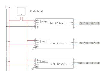
Only use the open push button WITHOUT an indicator light. Max. cable length between each driver: 65 ft 7 in. (20 m)
